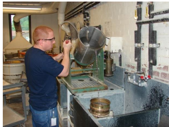
Mechanical Wash Method
