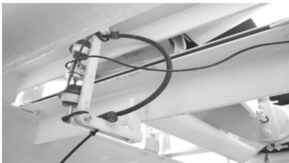
Weigh Bridge Load Cell
