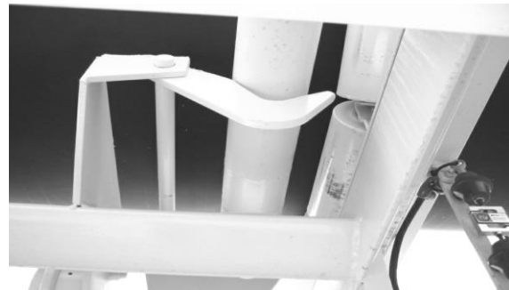
Hanging Weight on Weigh-bridge
