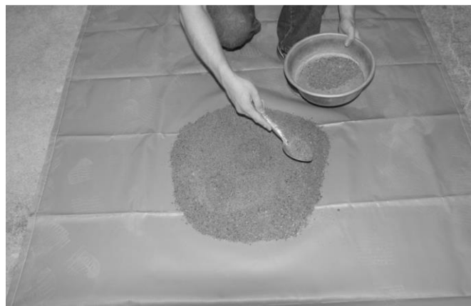
Figure 4 – Miniature Stockpile Method on a canvas blanket or tear resistant tarp.
