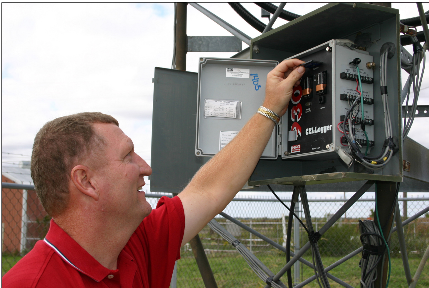
Tim VanDyke, division chair for technology reads a meter that measures wind speeds on campus. Through the wind feasibility study, it was determined that LLC has high Class II wind speeds.
