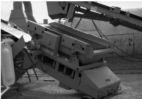
Dryer-Drum Cold Elevator Scalping Screen
