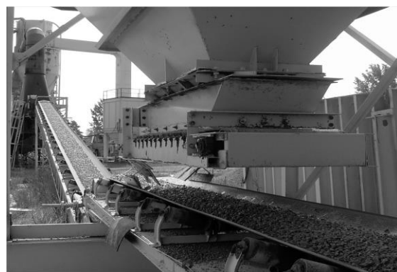
Cold elevator leading into the drier
