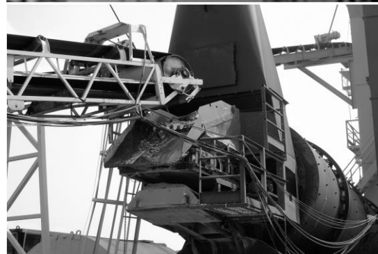
Batch Plant Slinger Belt, Scalping Screen and Scalping Material Diverter
