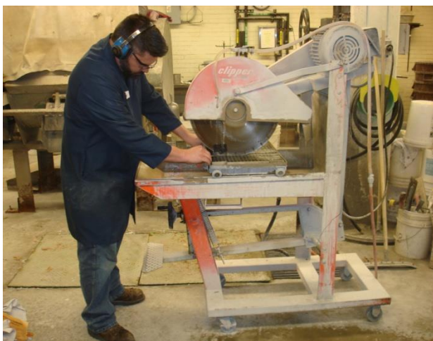
Sawing the samples
